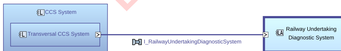
Figure 6 Context Diagram of Railway Undertaking Diagnostic System
