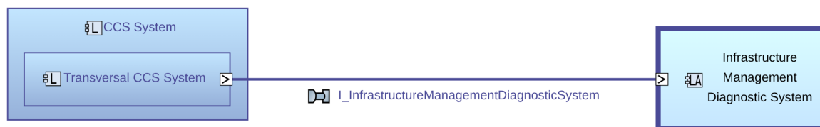
Figure 4 Context Diagram of Infrastructure Management Diagnostic System
